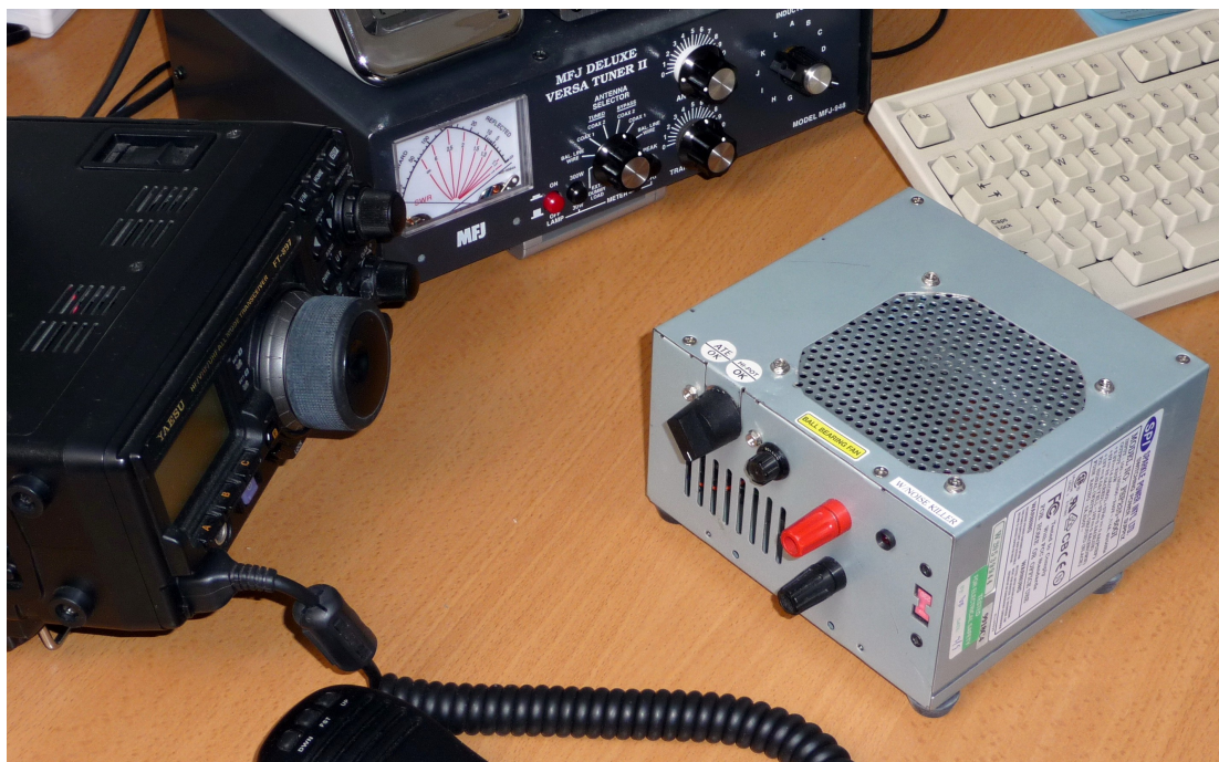
Figure 1 The finished junk box FT-817 power supply ready for operation
