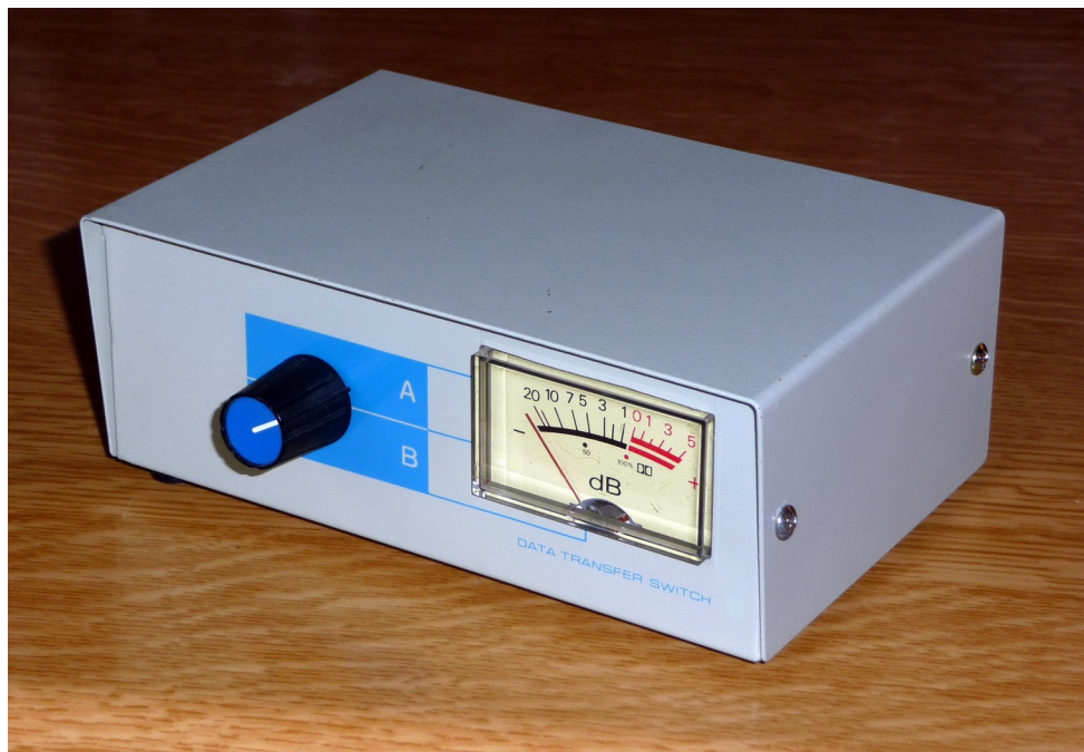
Figure 2 The finished RSRI built into a surplus parallel printer switch box
