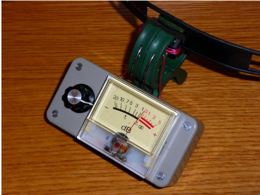
Figure 2 The RF clip meter clamped over one of the conductors of a 10m length of 450 ohm balanced twin feeder
