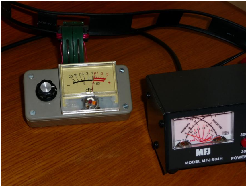
Figure 3 The RF clip meter and MFJ Travel Tuner indicating a maximum RF output of 10W during final tune-up prior to one of the 2010 RSGB 80m CC contests
